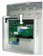
5. Push the PCIe card holder in the direction of the PCIe card and secure this with the marked screw.
