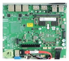
6.2 Installing and removing a memory module
