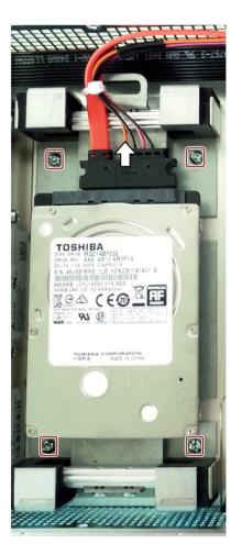
4. Detach the hard disk from the base plate. Remove the four screws that connect the hard disk and the base plate.
