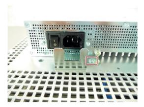
3. Insert the power cable into the socket and fasten the power plug fastener with the marked screw.
