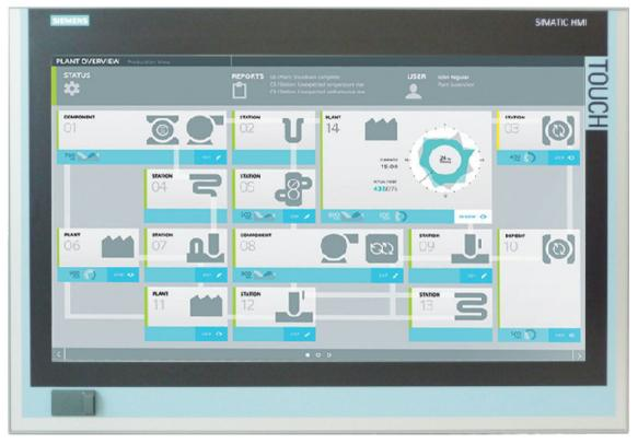
Figure 1-1 Device with resistive single-touch screen
