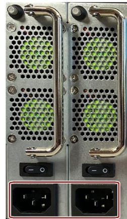
Redundant power supply (350 W)
