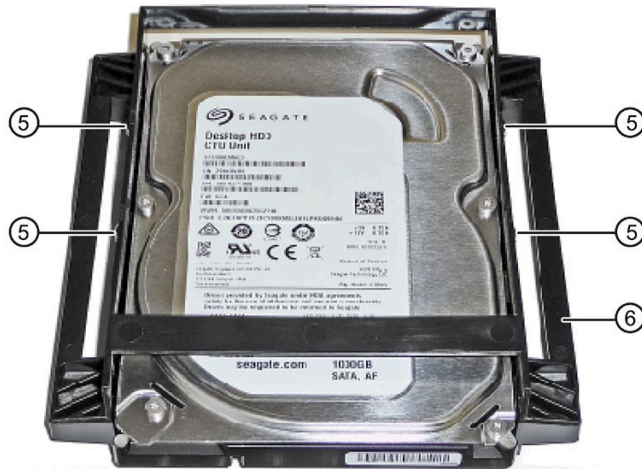
Drive cage with 3.5" HDD
