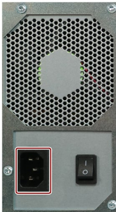
Single power supply (400 W)
