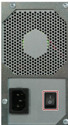
Single power supply (400 W)
